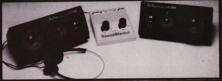
Everyone knows that the Amiga has excellent sound capabilities. Televisions and monitors do not produce hi-fi sound output, so until now it has been impossible to connect your Amiga to an amplifier to appreciate the sound quality. The Amiga SOUNDBLASTER is a small amplifier that comes complete with two high quality 50 watt 3-way speakers. It is easily connected to your Amiga and adds a new dimension to all your games.
