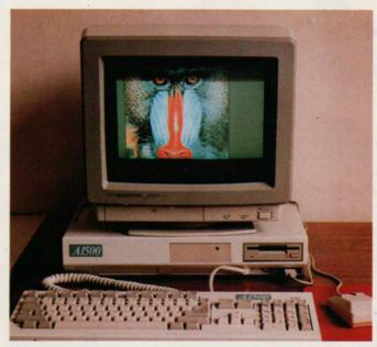
The A1500, an adaptation of the A500, offers a separate keyboard and brings disk drives and joystick ports to the front.
